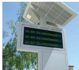
To combine transport and sustainability, some of the screens are fed with solar energy.
